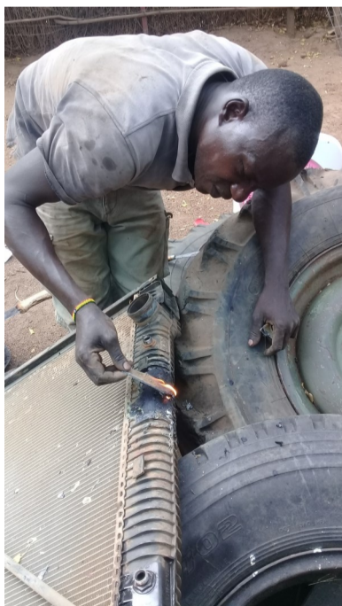
Stephen Okello uses plastic and fire to repair a hole in the radiator of the green UniMog Tipper Lorry.
